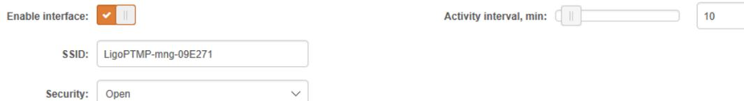
The screenshot shows a configuration interface with a toggle switch for 'Enable interface' (checked), an 'Activity interval, min:' slider set to 10, an 'SSID' input field containing 'LigoPTMP-mng-09E271', and a 'Security' dropdown menu set to 'Open'.
