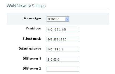
**IP** address - specify static IP address for CPE WAN interface.
