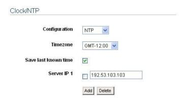
**Configuration** – choose the system clock configuration mode [NTP/Manual].
