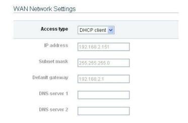
After setting the CPE access type as DHCP client and rebooting the device, the current IP settings received from the DHCP server will be displayed at the disabled entry fields of the WAN networks settings.
