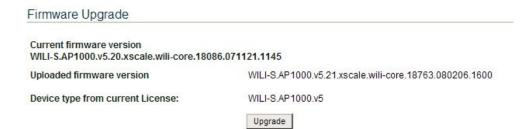
**Upgrade** – upgrade device with the uploaded image and reboot the system.
