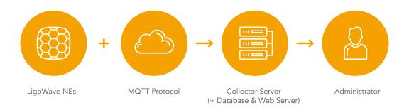
LigoWave NEs (Infinity, DLB, or PTP) gathers and processes data from connected client devices. It is then sent to a Data Collector Server using the MQTT Protocol. This server also hosts the database and the web server, which are used for storing device inventory data, config, and stats, and for the user interface respectively. From here, data travels to the administrator to be used as insights into network status, performance, and other metrics.
