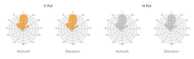
Frequency Range 5.1-5.9GHz 15dBi Gain Polarization Dual Linear Cross-Pol Isolation 21dBi VSWR <1.4 35° Azimuth Beamwidth (H pol) 35° Azimuth Beamwidth (V pol) 35° Elevation Beamwidth
