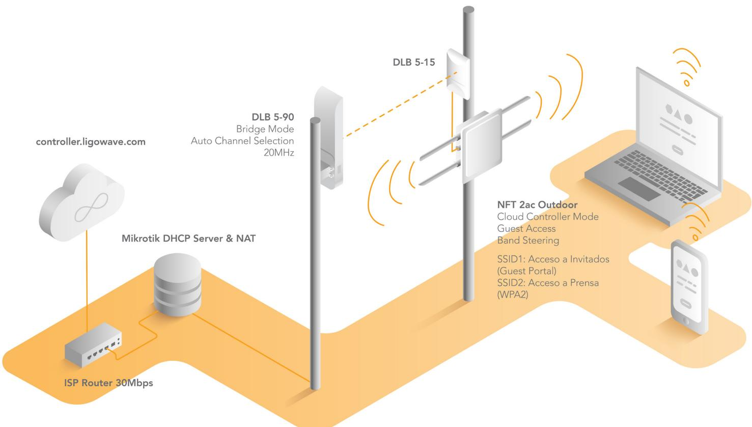
**Wireless backhaul and Wi-Fi network topology:** internet access was provided via the ISP's router, which was hooked up to a DLB 5-90 wireless base station operating as a PTMP backhaul bridge. It linked 5x DLB 5-15 client devices, each of which was connected to an NFT 2ac Outdoor Wi-Fi access point. The maximum distance between the base station and the client devices was 500 meters.
