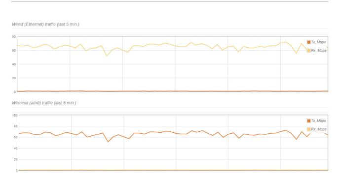
Throughput information on the base-station user interface. Single direction traffic is generated from AP to CPEs.
