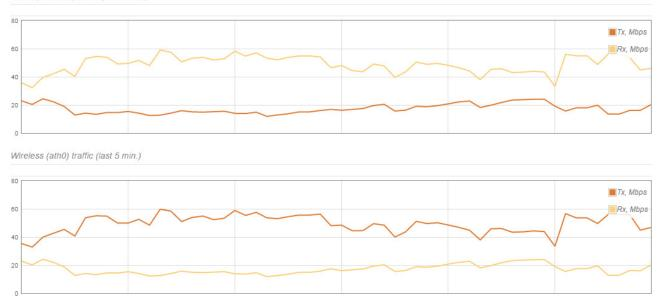
Throughput information on the base-station user interface. Bidirectional traffic is generated from AP to CPEs.
