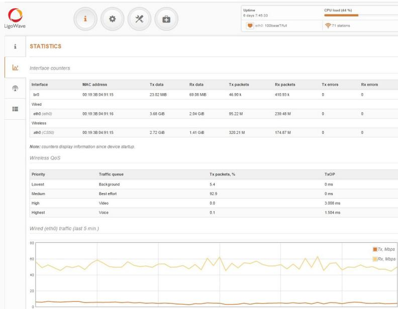
This image is a screenshot of AP's statistics window, where an administrator can view a real time throughput graph. At that moment the aggregated throughput was about 60 Mbps and most of it was in a direction from AP to CPE (received on Ethernet port). Even with many active stations, the GUI responsiveness was fast and reliable.
