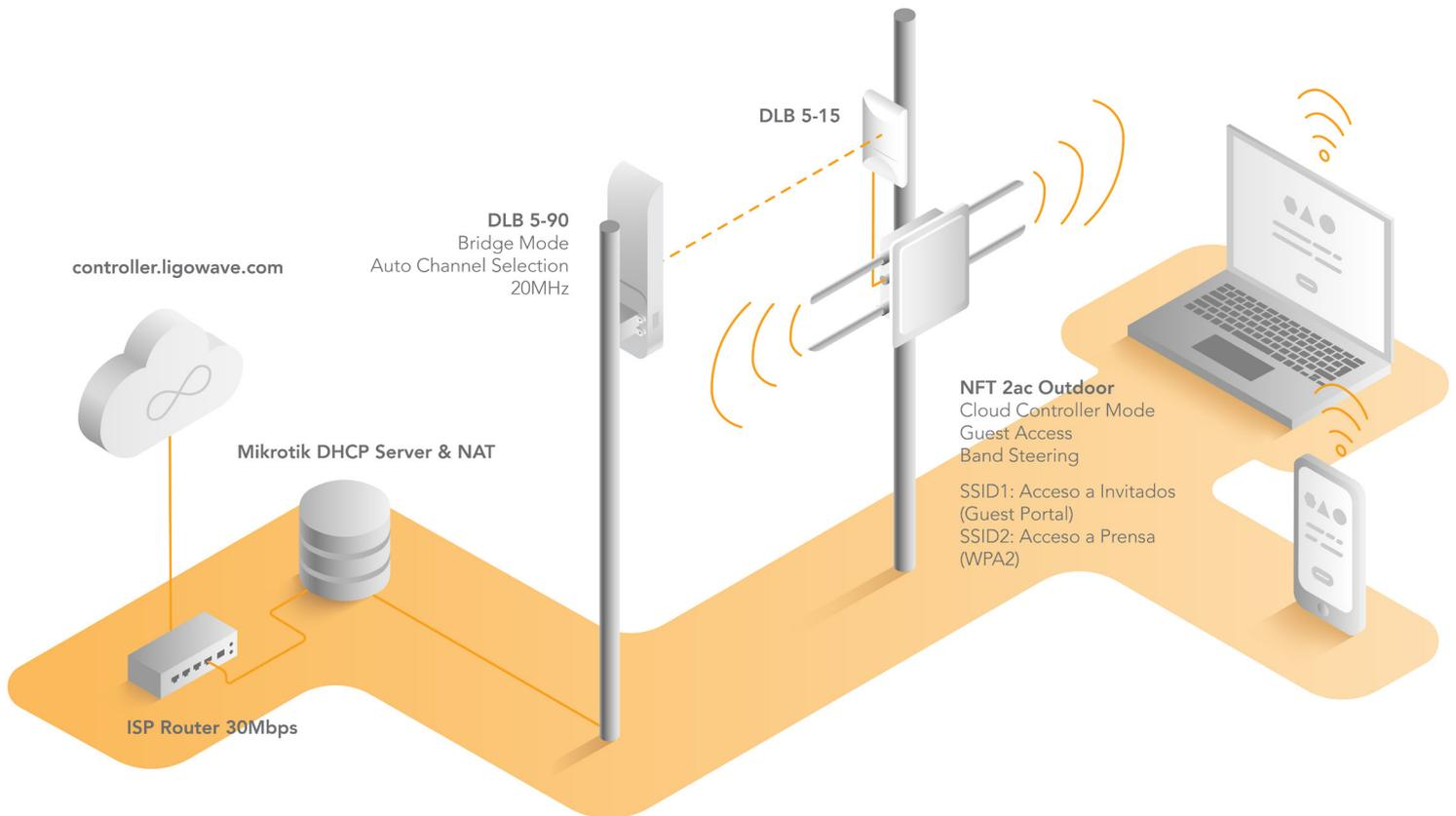
*Wireless backhaul and Wi-Fi network topology: internet access was provided via the ISP's router, which was hooked up to a DLB 5-90 wireless base station operating as a PTMP backhaul bridge. It linked 5x DLB 5-15 client devices, each of which was connected to an NFT 2ac Outdoor Wi-Fi access point. The maximum distance between the base station and the client devices was 500 meters.*
