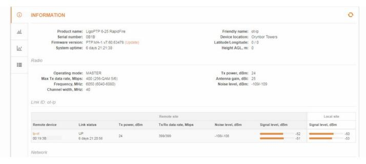
Low noise levels in the 6GHz band and-50dBm average signal level ensured good performance and stable connectivity.
