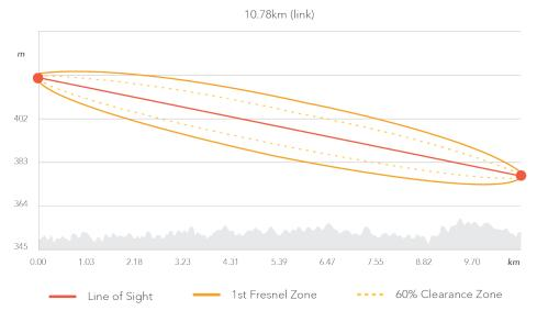
Link path profile showing a downward wireless link. It does not include buildings, but is otherwise with clear line of sight.
