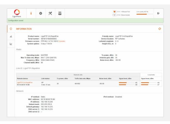
The GUI screenshot above illustrates the main statistical information about the link. The signal level is in the -65 dBm range, which will not allow it to achieve the maximum capacity possible. To improve that, higher gain antennas are necessary.
