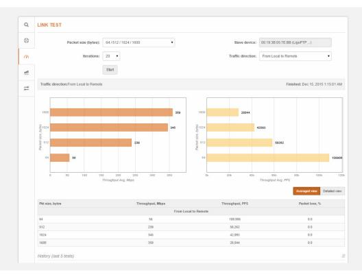
A screenshot from the link test tool indicates the max capacity of 350 Mbps with 1600 byte packets and a PPS of 108,000 with 64 byte packets.
