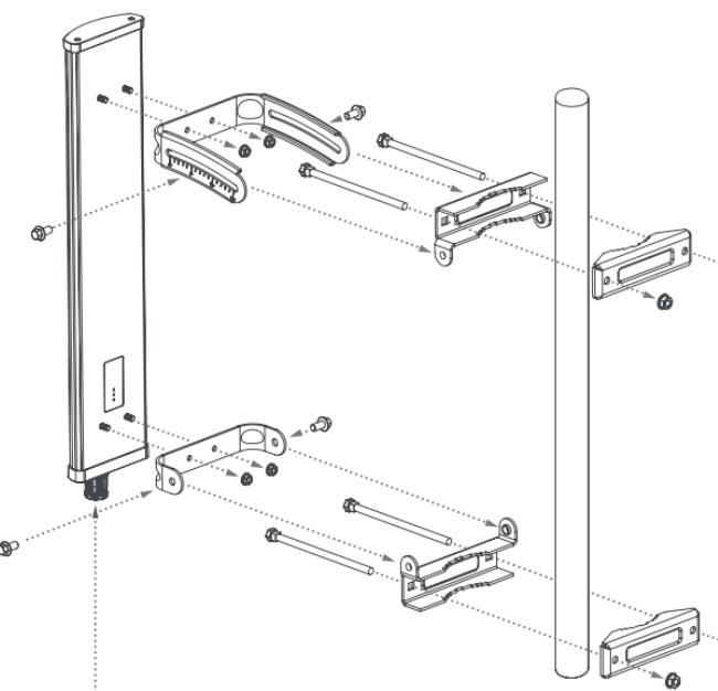
Device cable gland must be positioned vertically downwards to protect it against water ingress.
