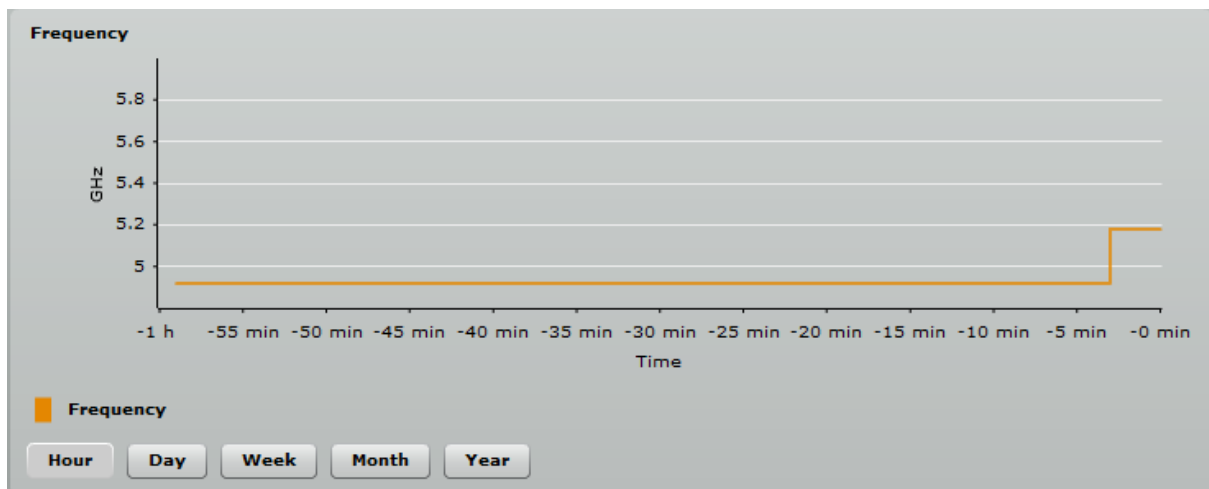
Figure 27 – Frequency Graph at which PTP Link is Operating
