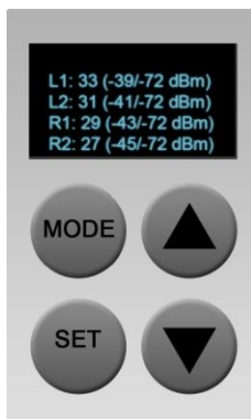
Figure 23 – Antenna Alignment Tool on OLED
