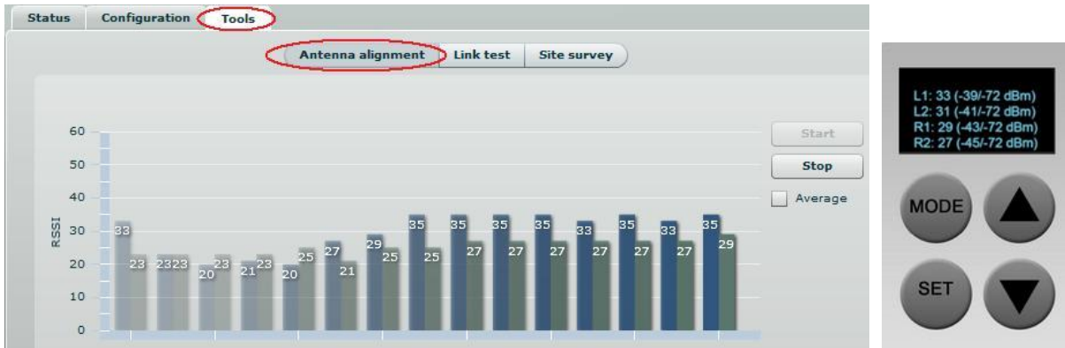
Figure 2 – Antenna Alignment Tool on Web and OLED.
