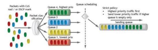
• **WRR** - with this scheduling, a set number of packets from each queue is transmitted, in a round robin algorithm. The higher queue's priority, more packets are transmitted in as the algorithm cycles through the queues in turn. This method guarantees that every queue receives some attention from the port for transmitting packets.
