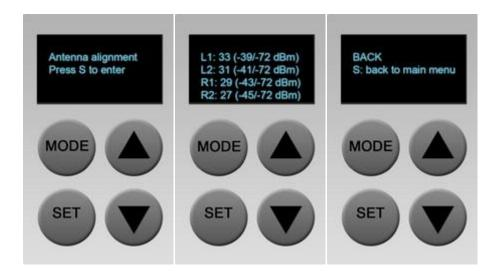
L1, L2 stands for local unit antenna 1 and antenna 2.
