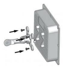
**Step 5.** Attach the second part of the mounting bracket to the wall using screws (not included) as displayed below:
