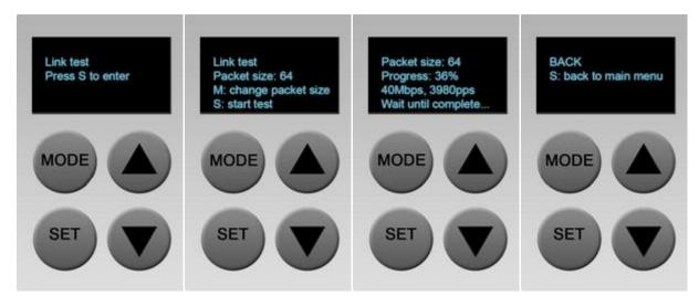
If PTP link is not established, the Link test menu displays the corresponding message "PTP connection is lost".
