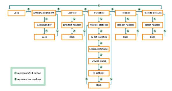
The following diagram represents OLED menu structure and navigation:
