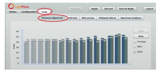
Antenna Alignment on OLED interface:
