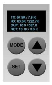
If the statistics value length is high and can't fit into the OLED's display, the value shall be divided by  $10^3$ ,  $10^6$  or  $10^9$  and the additional letter K, M or G shall be added then (e.g. TX: 40K/234M)
