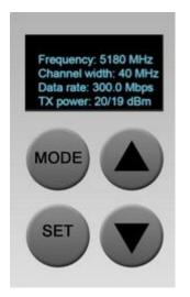
If the statistics value length is high and can't fit into the OLED's display, the value shall be divided by  $10^3$ ,  $10^6$  or  $10^9$  and the additional letter K, M or G shall be added then (e.g. TX: 40K/234M)
