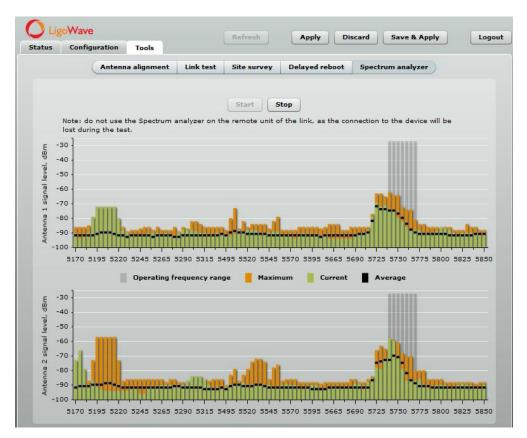
**Operating frequency range** – displays the channel frequency range at which the particular LigoPTP UNITY is operating currently.
