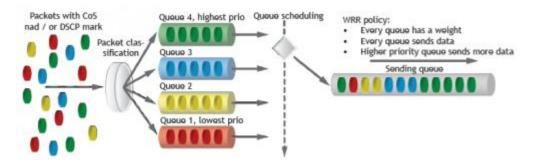
**QoS mapping precendence** - select the QoS mapping priority either L2 (802.1p) or L3 (DSCP). This option is available only if both types of QoS are enabled.
