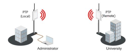
From the point of view of the administrator the **Local unit** is the one with the direct connection to the Web management interface and the **Remote unit** is the one which is connected to the Local unit in PTP link. The concept of the Local unit and the Remote unit is not related to the operating mode (Master or Slave). This terminology will be used throughout the manual, particularly in the description of statistics.
