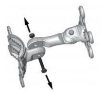
**Step 4.** Attach the following part of the mounting bracket to the LigoPTP UNITY unit with 4 screws as displayed below:
