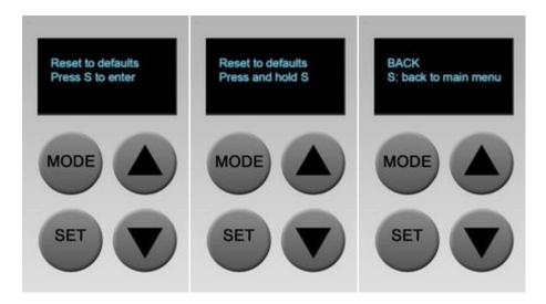
To return to the upper level menu, use an arrow key as a Back button and then press SET (S) key.
